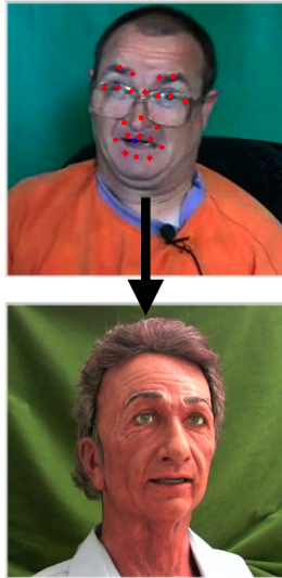
Fig. 3. 22 facial feature points from the original video are directly mapped onto motors on the robot, to create naturalistic movement.
